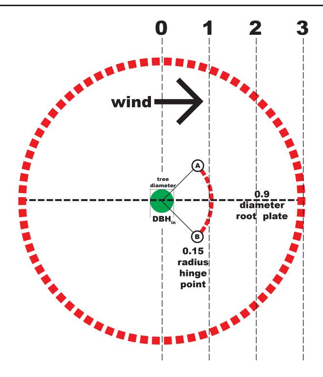
Figure 19: View from above of a tree root plate surrounding a tree of a set diameter (DBH<sub>in</sub>).
