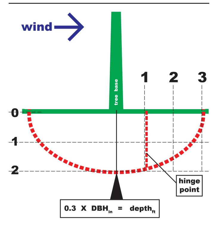
Figure 18: Side view of a tree root plate area showing root plate depth and location of hinge point in an unconstraining soil.
