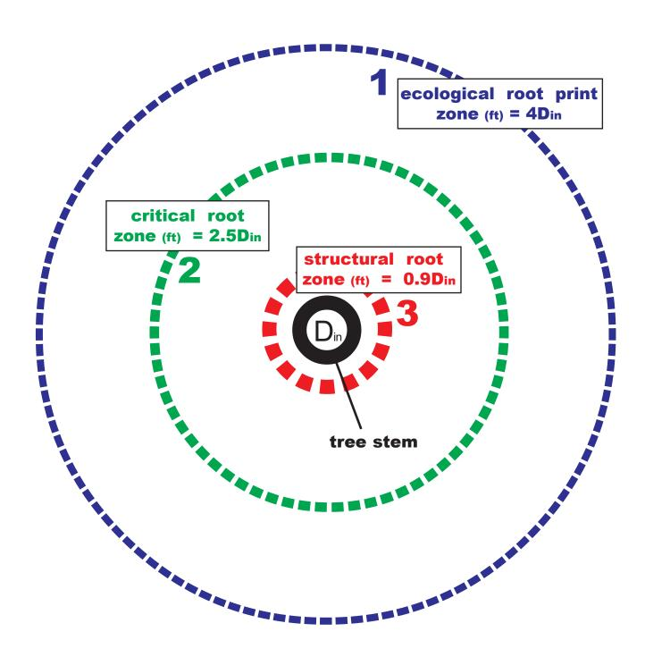
Figure 9: Site view from above a tree stem showing three different rooting areas and their limiting distance away from a tree.
