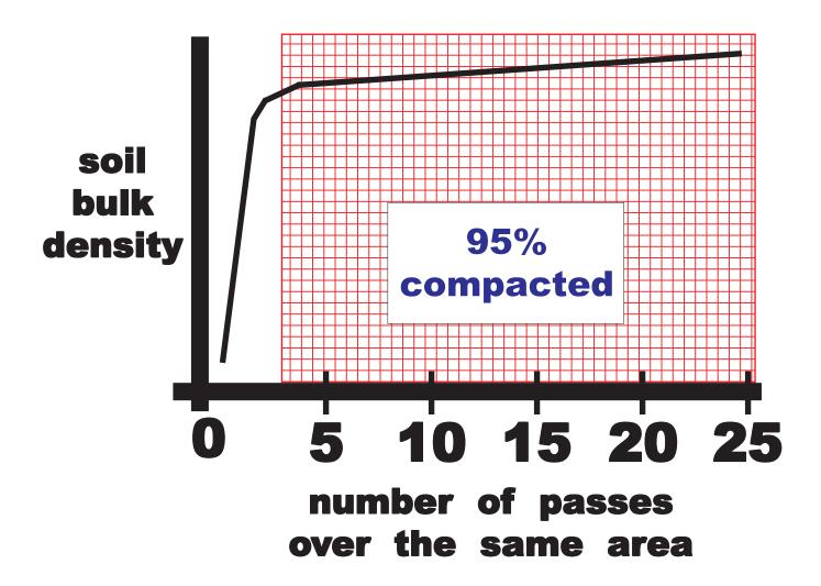
Figure 29: The number of passes over the same square inch of soil to increase bulk density (compact soil) to 95% of what it can be compacted.
