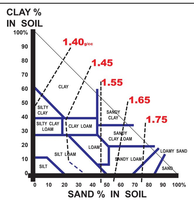
Figure 30: Soil textures classifications based upon sand and clay proportions, and dotted lines showing root-limiting bulk densities (g/cc). Values equal to or greater than listed density value (to the right of) will significantly constrain tree root growth.
