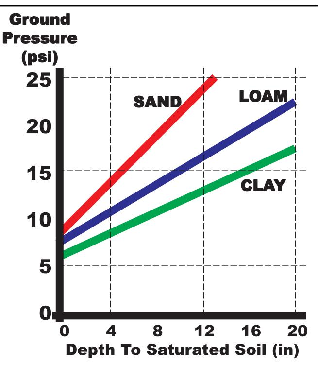
Figure 33: Soil rutting potential on wet soils under development activities. Ground pressure (psi) for vehicles: rubber tires = 20+; crawler track = 12+; and, floatation tires = 6+.
