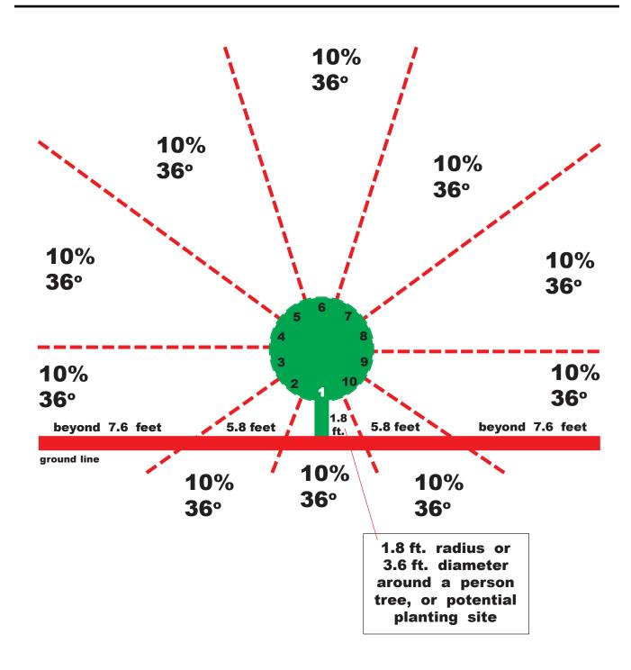
Figure 38: Diagram showing how heat loading can be estimated on a site using a combined and averaged view-factor for hardscapes / non-evaporative surfaces from 10 equal (36°) observation angles.
