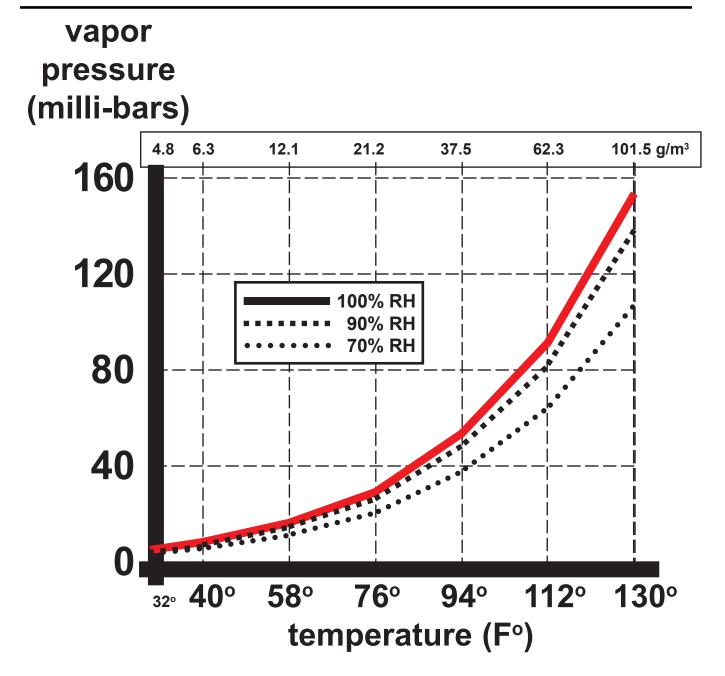
Figure 9: Saturated vapor pressure of water in atmosphere (100% relative humidity), the most water vapor normally found in air above liquid water. Also shown are 90% and 70% relative humidity (RH). The box over the graph contains the actual amount of water (vapor density in grams per cubic meter) in air for each temperature. (value approximations derived from Tabata, 1973)
