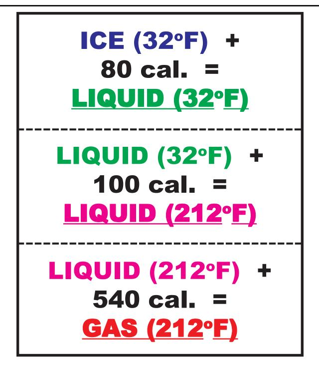
Figure 12: Water physical state changes with energy added (cal. = calories).
