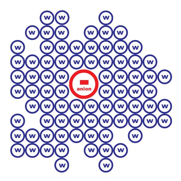
Figure 8: Two-dimensional diagram of water molecules surrounding an ion with a negative charge generating a hydration sphere effectively increasing ionic size. The partial positive charges on the water molecules line-up facing toward the negative ion.
