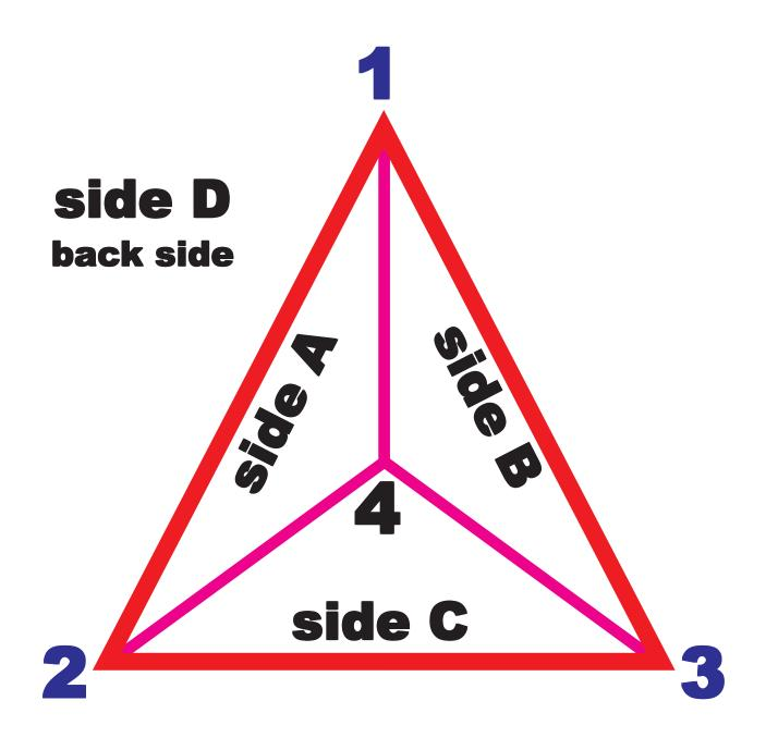
Figure 4: Oxygen bond attachment geometry is in the form of a tetrahedron with four corners (1-4) and four sides (A-D), only two corners can be filled with hydrogens.
