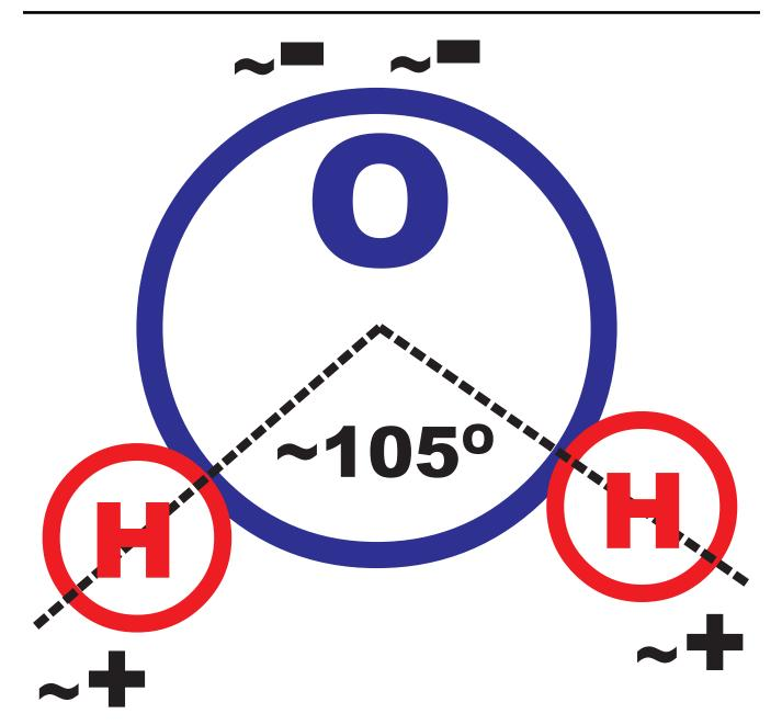
Figure 5: Diagram of water molecule with oxygen (O) and two hydrogen (H) atoms. Hydrogen atoms are always separated by ~105° as they glide over the oxygen perimeter, never on opposite sides. Oxygen draws electrons away from hydrogens generating a polar molecule with partial negative charges (~-) on the oxygen side and partial positive charges (~+) on the hydrogen side.
