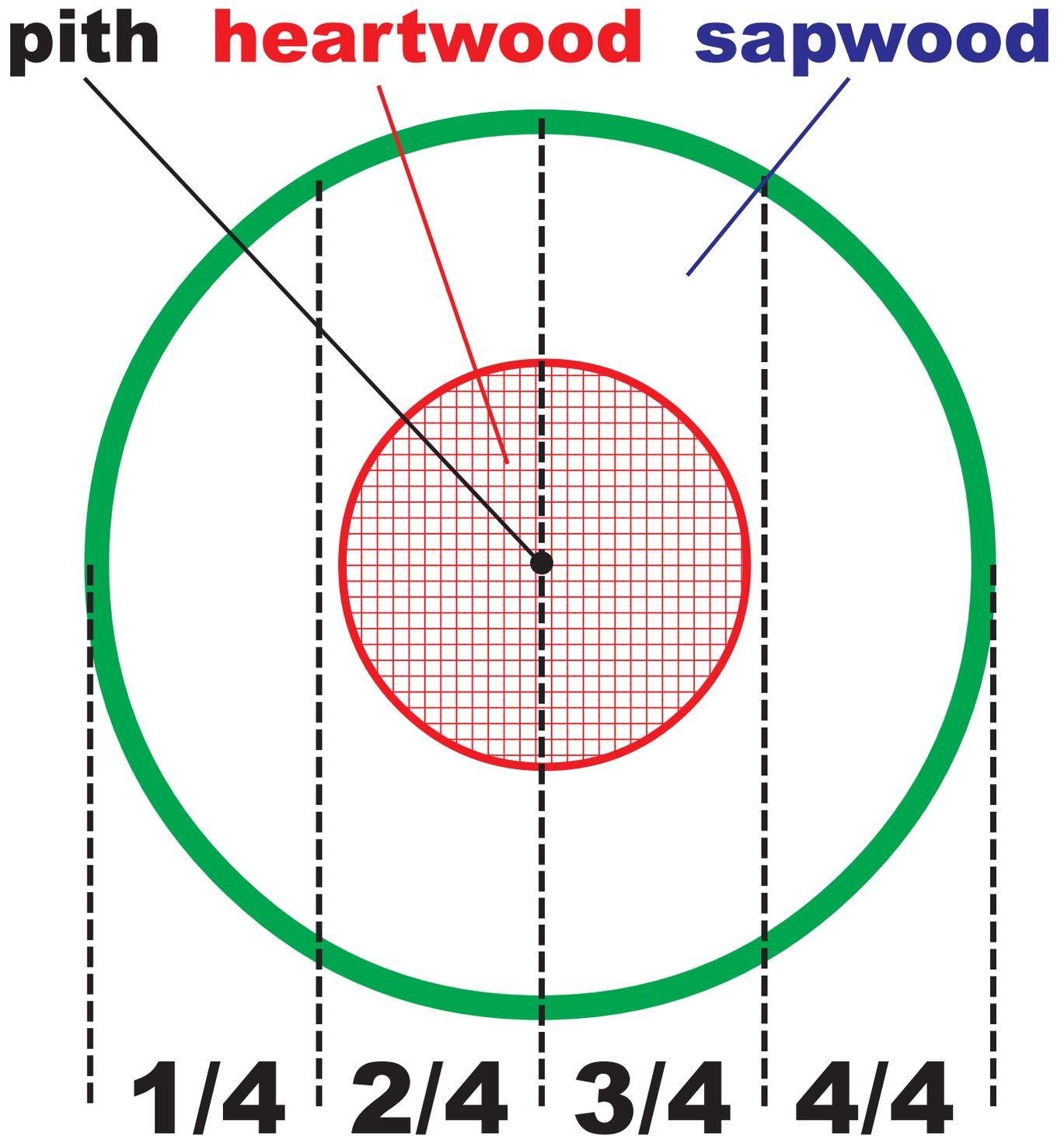
Figure 14: Coder Heartwood Exposure on Pruning Wounds Assessment for trees pruned, tipped or topped showing heartwood exposure >1/4 wound diameter.
