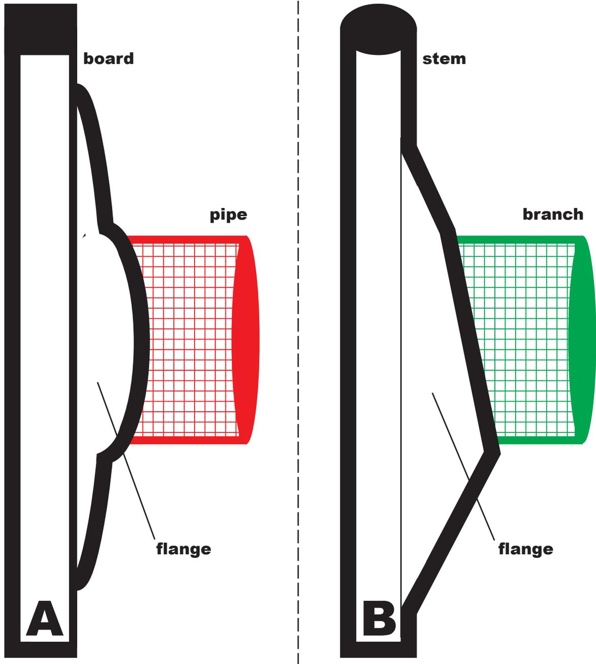
Figure 6: Descriptive model of a pipe held onto a board with a flange (A), and a branch held onto a stem with a combined tissue area acting as a flange (B).
