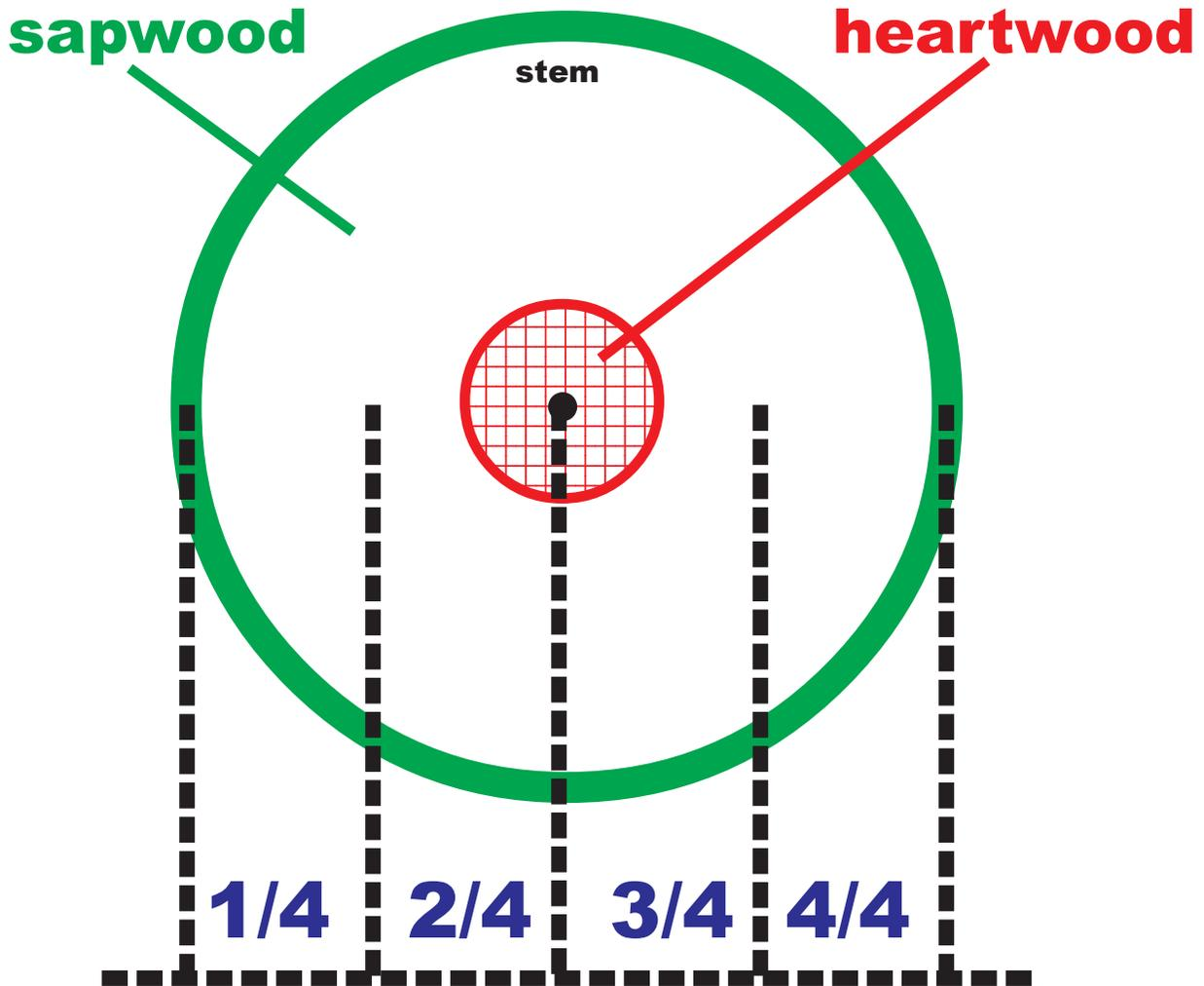
Figure 48: Diagram showing how heartwood size in a branch or stem can be measured. Heartwood exposure is described as a percent or fraction of total branch or stem diameter. In this case heartwood comprises 1/4 of stem diameter.
