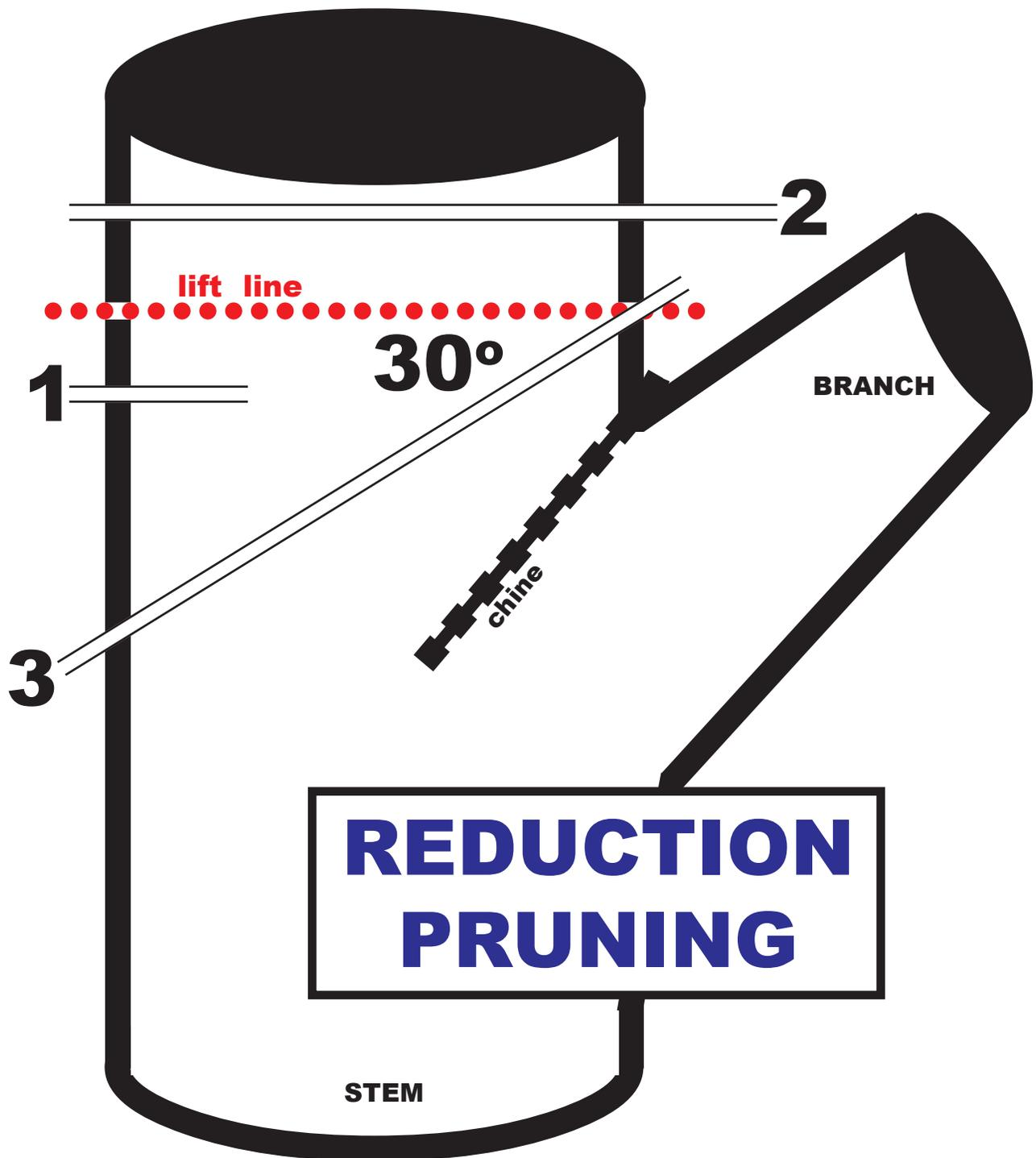
Figure 29: Diagram of confluence with three cut lines, numbered in order, for a reduction pruning prescription. Note the final (3<sup>rd</sup>) cut is at 30° down angle from the branch side of the lift line. The down angle is not dependent upon the chine or branch angle.
