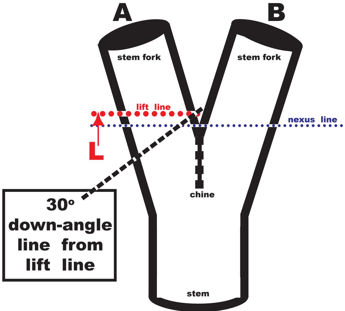
Figure 30: Forked stem with target lines established to initiate a reduction pruning prescription on stem fork A (left fork). Note lift line is made parallel to and above nexus line which is perpendicular to the longitudinal axis of the main stem before the fork and anchored at top of confluence. L distance upward is  $1/9X$  stem fork A diameter, or at least  $3X$  saw kerf.
