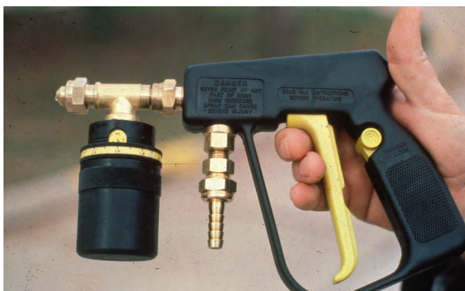
Figure 66. A spot gun that can be attached to a backpack sprayer to deliver small herbicide (1-4 ml undiluted for some herbicides) doses in a grid pattern or at the base of woody competition
