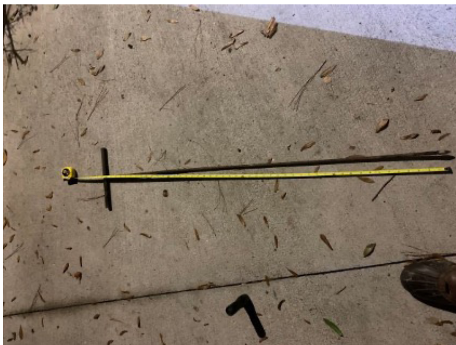
Photo 4: A drain tile probe can be used to see if a hardpan has developed on a site.
