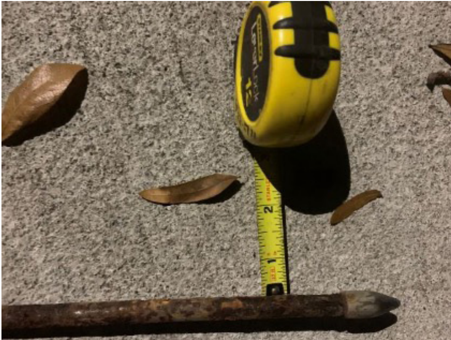
Photo 5: The drain tile probe metal rod has less than ½ inch diameter and a pointed end.
