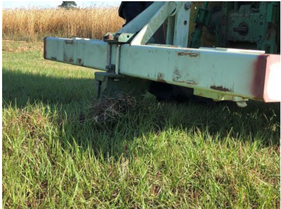
Photo 2: The toothed ripper over 18 inches deep in the soil.
