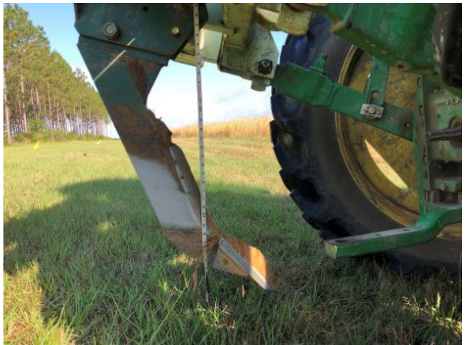
Photo 1: A ripper tool with a “tooth” at the bottom approximately 2 ft long is shown. The ripper tooth provides some soil fracture and better tillage but not as much as the wings of a subsoiling tool. Common agricultural ripper tools have no tooth, just a straight shank. These do not provide as much soil fracture and may be used closer to planting time.
